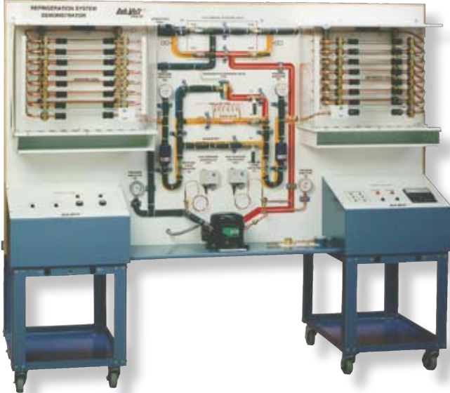
Model 3400: Refrigeration System Demonstrator
